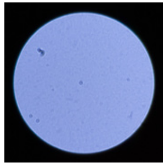
Point source lens fingerprints created at full aperture, defocused to project a disc – top left, a Sigma 70mm f2.8 macro showing high quality final polishing but needing a clean; top right, Sigma 18-250mm zoom shows rings formed by the irregular surfaces of moulded aspheric elements, and one dust particle. Below left, the diffraction coating pattern of a Minolta Portrayer 3 soft focus filter revealed, on a 70-210mm f4 AF zoom. Below right, the lens-shaped distorted ellipse projected by a 50mm f1.4 Sony lens wide open, corner of shot.
