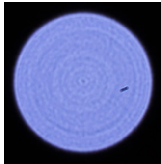
Point source lens fingerprints created at full aperture, defocused to project a disc – top left, a Sigma 70mm f2.8 macro showing high quality final polishing but needing a clean; top right, Sigma 18-250mm zoom shows rings formed by the irregular surfaces of moulded aspheric elements, and one dust particle. Below left, the diffraction coating pattern of a Minolta Portrayer 3 soft focus filter revealed, on a 70-210mm f4 AF zoom. Below right, the lens-shaped distorted ellipse projected by a 50mm f1.4 Sony lens wide open, corner of shot.
