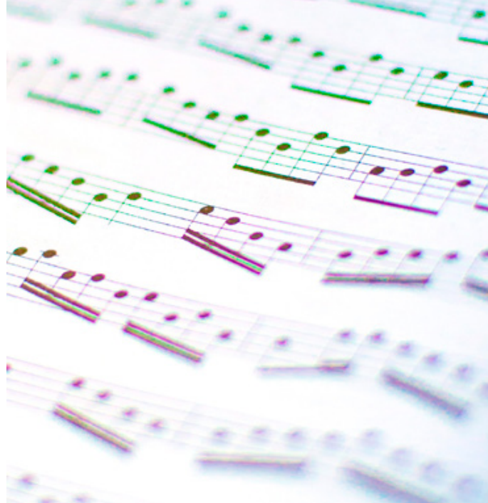
Above: by boosting Saturation and Vibrance, the colour bokeh shift of a Voigtlander 58mm f1.4 at f2 is seen clearly.
